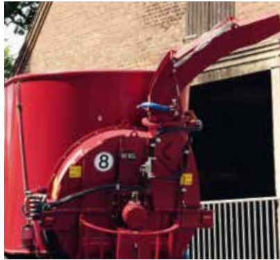
ROTATING, FOLDING TOWER Compact rotating ejector for flexible throwing on all sides.
