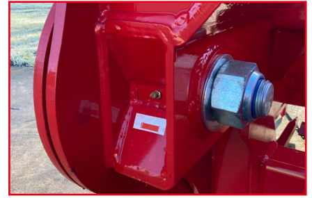
Stable pivot points with \varnothing up to 60 mm for 130 series
