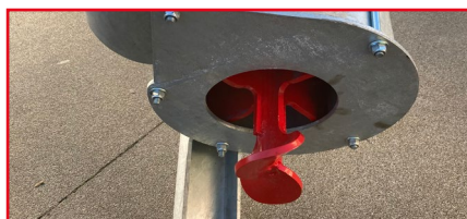
The cutting rotor cuts silage and other matter found in slurry. It prevents blockages and produces more homogeneous slurry.
